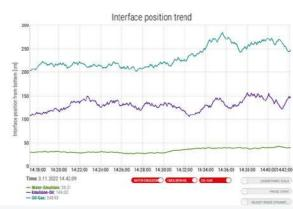
Electrical Tomography provides a real-time permittivity/conductivity profile which generates an overall picture of the actual process levels. With the SeeBeyond you can reliably identify when the changes happen. The interpretation is based on unique actual real-time data.
